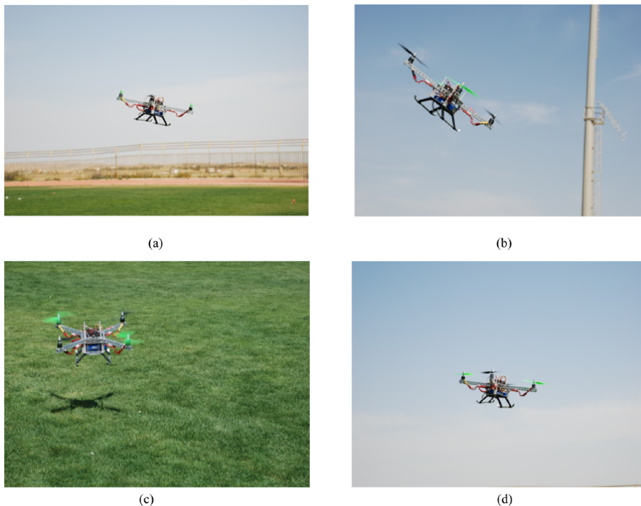
Figure 15 Snapshots of the quad-rotor in flight demonstrating the difference in behaviour between the LQR and the MRAC controller: (a) the LQR responses at low altitude using a single faulty bearing; (b) the LQR responses at high altitude using a single faulty bearing; (c) the MRAC responses at low altitude using a single faulty bearing and (d) the MRAC responses at high altitude using a single faulty bearing (see online version for colours)
