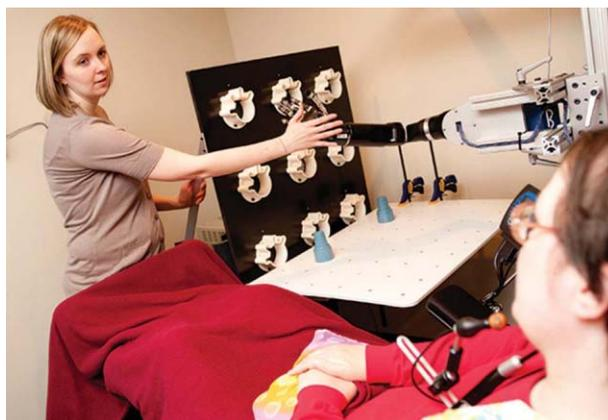
**[FIG2]** Jan Scheuermann (right) reaches out with the thought-controlled robot arm to touch Jennifer Collinger's hand. (Photo courtesy of the University of Pittsburgh Medical Center.)
