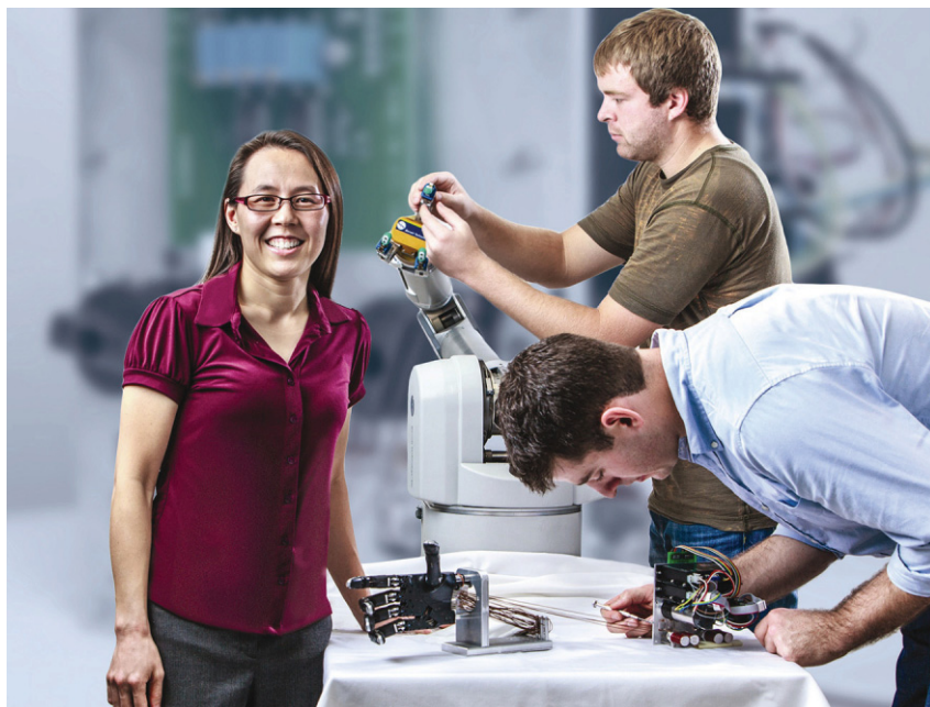
[FIG1] Dr. Santos (left) is shown with Biomechatronics Lab members Ryan Manis (right, back) and Randall Hellman. Ryan is mounting a tactile sensor on a robot hand while Randall is adjusting the lab’s custom remote actuation system for tendon-driven mechanisms. (Photo courtesy of ASU Magazine and Dan Vermillion of Vermillion Studio.)
