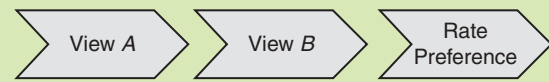
[FIG4] Pair comparison rating cycle: the subject watches video sequence A , then watches video sequence B , and rates B relative to A .
