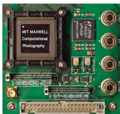
[FIG3] A printed circuit board containing MIT’s “Maxwell” computational photography processor. (Photo courtesy of MIT.)
